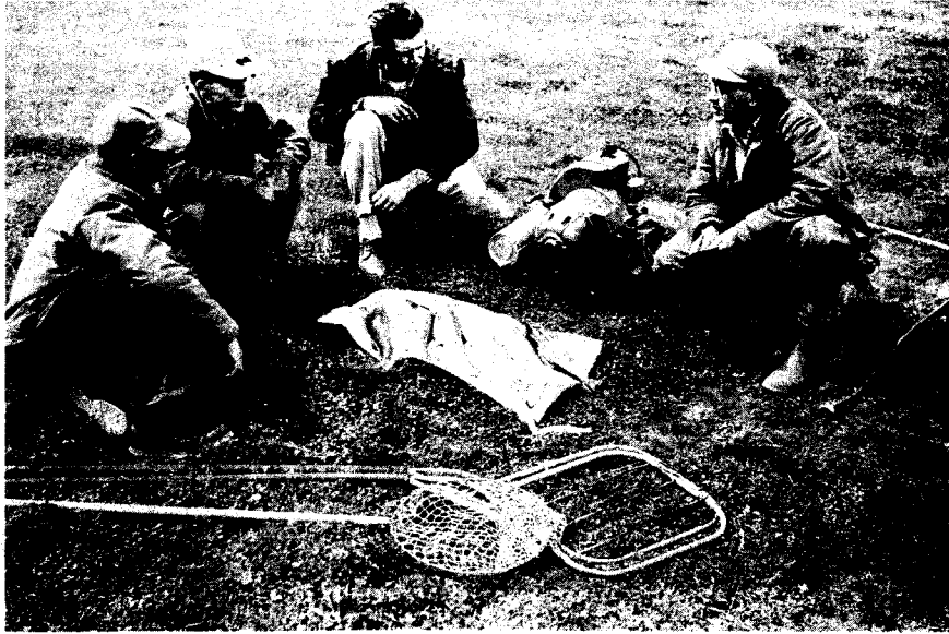
Plate 36. Dip net, electrodes and 2500 watt direct current electrical shocker used to collect fish from fishways.
